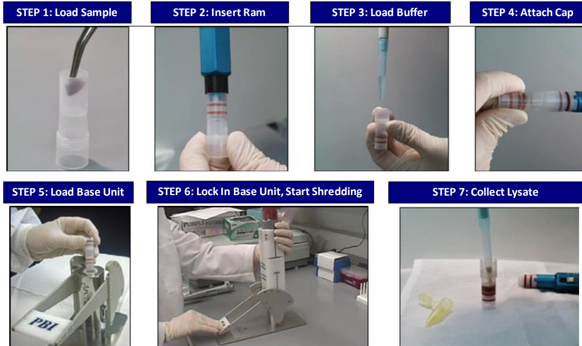
Figure 17 GENERAL STEPS FOR USING THE SHREDDER SG3
